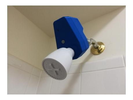
QiQi is a Bluetooth Low Energy (BLE) Shower Controller that allows you to remotely control your shower using your mobile phone or tablet device. Using the QiQi mobile app, you can remotely warm up your shower. Pressing the button in the app opens the valve, and the temperature sensor inside QiQi monitors the water temperature. When the water is hot QiQi closes the valve, and then alerts you on your phone that your shower is ready. No more \$\$ down the drain!!
